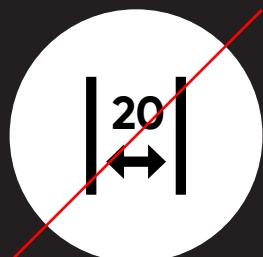
**Leave at least 20 cm of space around the machine for free air circulation and better performance. Do not cover the ventilation grids.**
